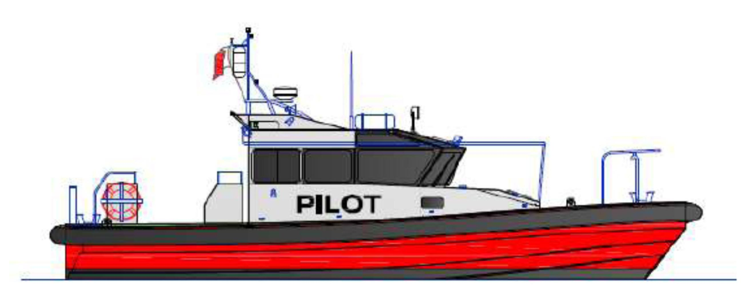
This Pilot Boat is one of a series of Fast Pilot Boat designs by Camarc. The double chine hull gives exceptional all-round seakeeping and has been proven on over 100 pilot boat craft in service worldwide.
